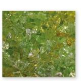
Recycled glass filter material that is much more effective than sand: it provides greater water purity and better water quality. Its smooth micro-surface has self- sterilizing and oxidizing properties, less soils with fats, lipids and biological growths. It helps to reduce the carcinogenic byproduct of chlorinated disinfectants, trichloramines. To regain approx. half the water is needed as for sand filters.
