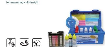
Our testers provide a more accurate definition of the measuring strips. Their use requires a reagent tablet, which results in the discoloration of the test sample depending on the degree of the parameters to be measured. By comparing the color and the scale you can easily read the result.
