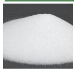
99.7% pure NaCl (table salt) in granular form. Recommended for the manually operated equipment's ion exchange resin charge's regeneration.
