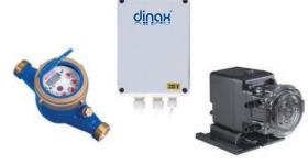
A quantity-proportional dosage device, consisting of a water meter with a built-in encoder, a Dinax Pump Control Module transducer and a Stenner pump. The equipment controls the dosing pump by impulses (according to the impulses of the water meter) which then precisely doses the disinfectant as a function of the make-up water quantity.
