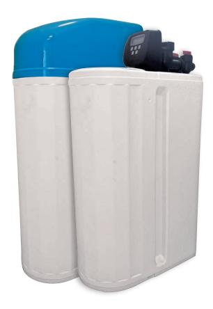
Our automatic softening equipment are quantity controlled, i.e. having a built-in water meter, and after the desired quantity is reached, the regeneration is automatically performed. Delays can be set for the time of regeneration.
