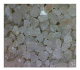
The burned quartz sand has far better filtration and cleaning capabilities than washed quartz sand. The reason for this is the firing process that burns out any organic contaminants. The burned quartz sand does not contain organic contamination and clay, in which bacteria and microorganisms could propagate.
