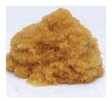
It is widely used for water softening, primarily for binding Ca- and Mg-ions. The charge replaces the cations of the water causing its hardness by Na- ions.
