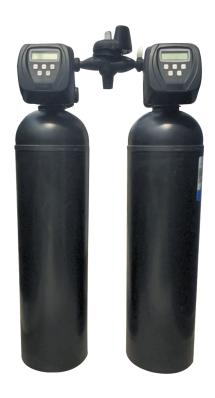
The equipment is automatically controlled, and ensures continuous soft water supply. Water softening is performed by the resin charge of one of the columns at a time, the other one functioning as a reserve standby unit.
