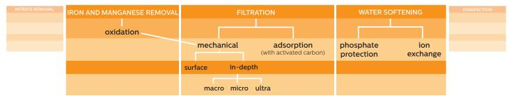
Surface filtration is based on the particles larger than the gap size of the filter medium are retained on the surface of the medium (a so-called sieve effect occurs). These filter elements can be cleaned and reused, if they get clogged.
